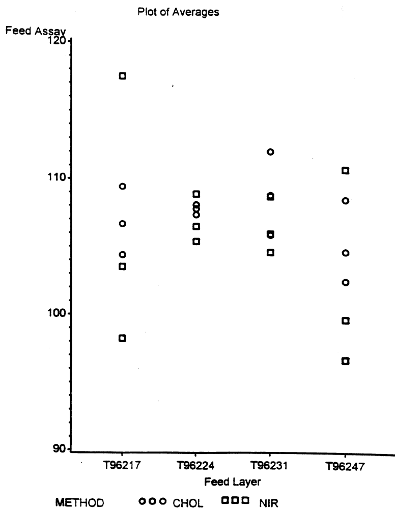
Fig. 5. Comparison of results for near-IR and cholate binding methods at the 1.5% level.
